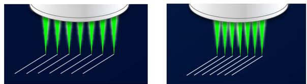
Spot distance easily changed by manual adjustment on unit
